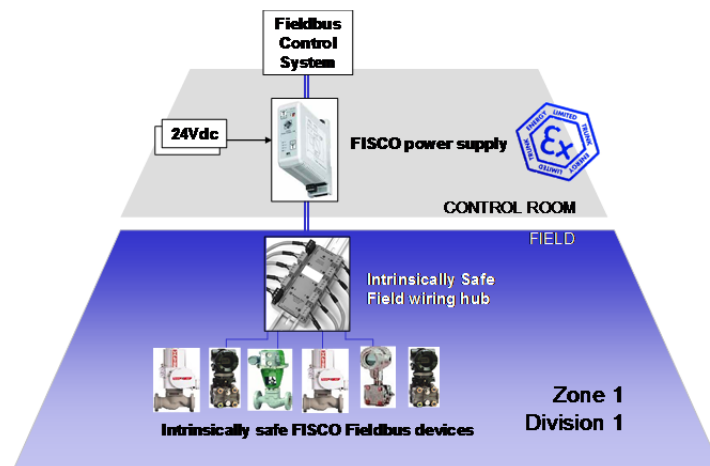
Figure 11.1: Typical FISCO segment
