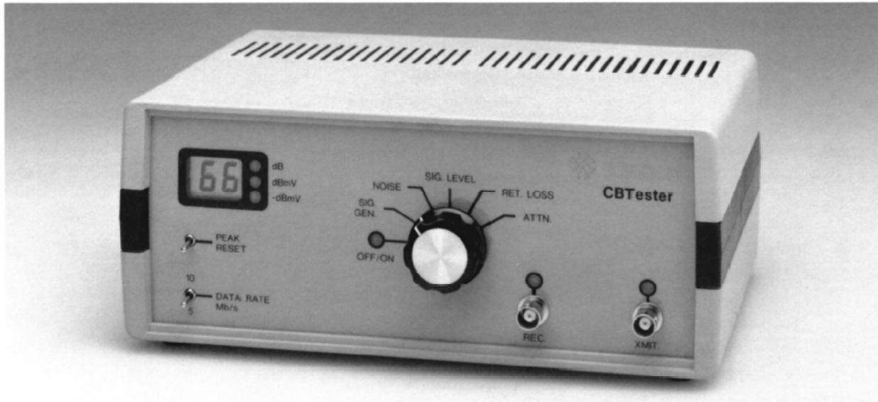
The Carrier-Band Tester, CB Tester, is a field service instrument designed specifically for the carrier-band network as it is defined in the IEEE-802.4 standards. The CB Tester is used for the network's cable system component qualification, cable-system installation and verification. The following types of measurements are made with the CB Tester:
