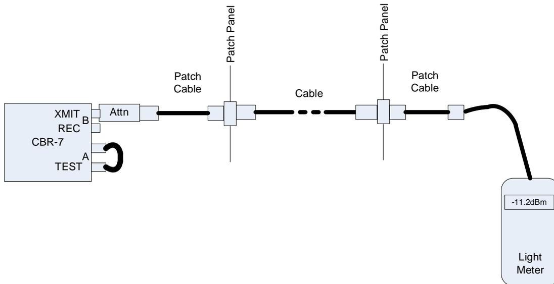
From the example above, if the light measured at the receiver is -11.2dBm then the **Measured Attenuation** of the optical components is:
