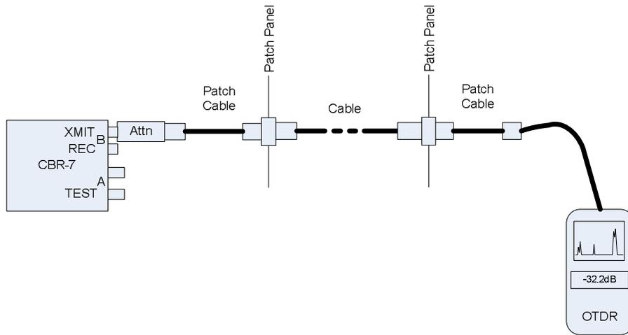
For proper operation of the CBR-7 repeaters over the fiber optic cable
