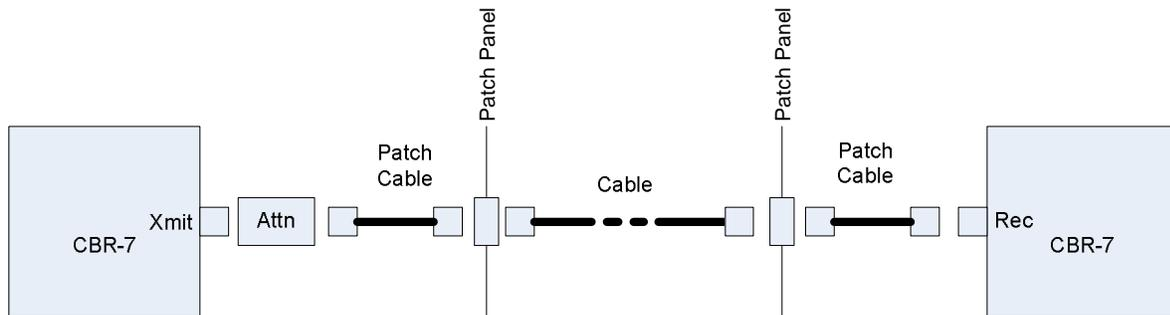
**The total attenuation (insertion loss) of optical components must be at least 15 dB but not more than 24 dB. If necessary, an attenuator must be used on the transmit side of the main fiber-optic cable.**
