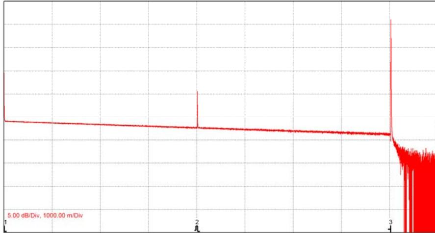
The top of the screen is at -10 dB. There are two reflections. One is at 4 km and the other at 8 km, at the end of the cable. The one at 4 km is 15 dB below the one at the end and it can be neglected since it is more than 10 dB below the reflection of interest at the end of the cable. The reflection at the end of the cable is at -14 dB. The return loss at the end of the cable due to this reflection is 14 dB, as seen from the other end of the cable where the measurement is made.
