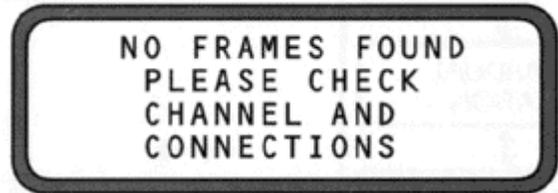
Figure 6. Display if Not Connected to Network
